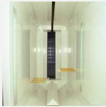
Automatic coating of complex-shaped objects is touchscreen interface enables performed using reciprocators and automated frontcomplete monitoring and rear carriages. management.
