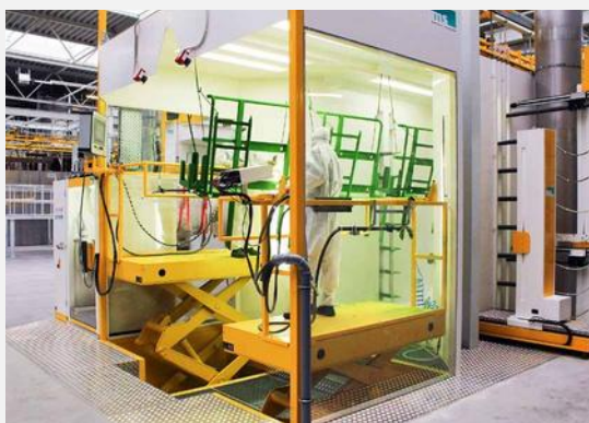
Manual coating area integrated with a scissor lift table
