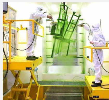
Flexibly supports powder coating for flat surfaces and large workpieces
