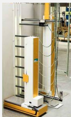
Automatic coating through combined X-Y-Z axis control
