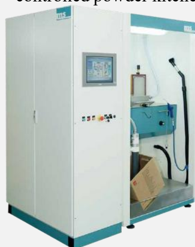
High-speed color change system integrated with PLC-controlled powder kitchen
